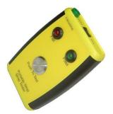
The unit is housed in a durable lightweight plastic moulded case with rubber hand grips on the side, making it ideal to use as a portable tester.
