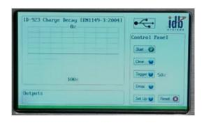
Charging of the test specimen is carried out by an induction effect and immediately under the test specimen, which is horizontally arranged, a field-electrode is positioned, without contacting the specimen, and a high-voltage is rapidly applied to the field-electrode.
